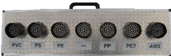
**Identification of different plastic types** is the result of a trained pattern recognition. After the measurement of the plastic sample the optical information (absorption bands of overtone- and combination vibrations) are processed by a neural network. The result of the calculation is a list of the most probable polymer type identified within a probability of 0 and 100%.
