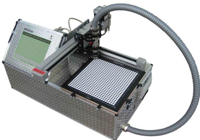
The **basic principle** of the method is the diffuse near infrared reflection spectroscopy whereby characteristic absorption behaviors of different polymer types are used in that spectral region. The polymer sample is radiated with a infrared light and the reflected light of the measuring focus is analyzed using a near infrared detector array.
