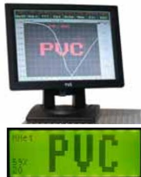
Additional connections like an USB-interface allow external data transfer. As an **optional feature** a LED array visualizing the identification result is available. (dimension in mm: 720 x 140 x 170, weight: 5 kg, power supply: 100-230 VAC, 50/60 Hz).
